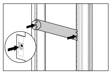
Figure 2-1. Measuring with the 2U template
